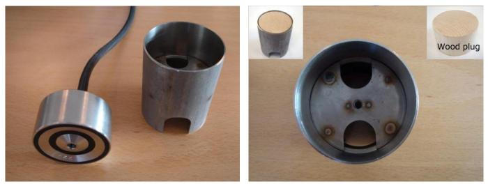
The sensor is delivered with a wood plug/cover to protect the hole when, for example, asphalt or concrete is being poured.
