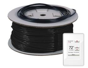
During installation the heat cable is tied directly to the re-mesh and embedded at least ½-inch below the surface. The thermal heating cable then heats and uses the concrete slab to store and distribute heat evenly throughout its intended area. In-Slab heating cable is affordable and can be installed under any type of flooring, including hardwood, carpet, laminates, and tile so you can enjoy radiant heated floors under any floor in your home.
