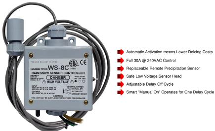
The **WS-8C** is primarily designed for gutter, downspout, and roof ice melting and small satellite antenna deicing. The totally sealed, low voltage, remote mount precipitation sensor allows the user to install the small sensor head in a downspout, the bottom of a gutter, or at the end of an antenna boom, up to 10' away, while keeping the main controller in a more convenient or protected location.
