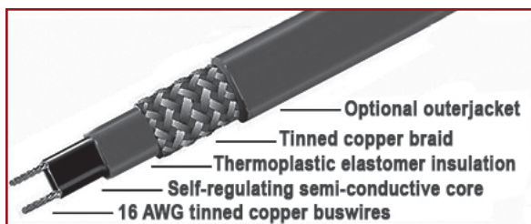
Cutaway view of Warmzone self-regulating heat trace cable.
