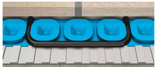
Thin set, the Prodeso membrane, heat cable and tile.
