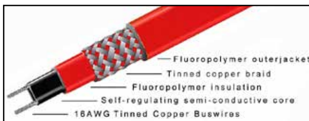
Cutaway view of PLSRS self-regulating heat trace cable.
