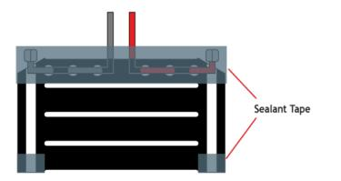
• Seal all connections by using the recommended sealant tape on the connector side of the element. Cut two pieces of tape slightly longer than the width of the element. Enclose the wire joints and strain relief connections with the two pieces of tape and firmly press the pieces together while overlapping the element to form a flat and smooth splice. Also use the recommended sealant tape to cover the bus braids at opposite end of the element. Refer to wiring diagram.
