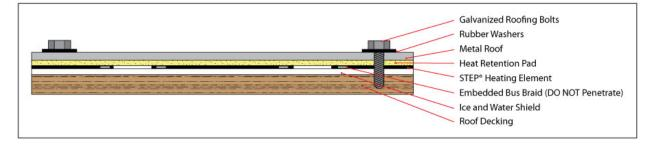
NOTE: Avoid overlap or contact between heating elements. DO NOT puncture the bus braids.
