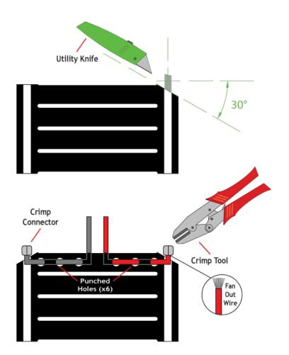
• Expose the bus braid by making an angled score in the plastic, front and back, and along the bus braid above the angled score with a utility knife. Bend the element where the cuts are made and pull off the corners to remove the surplus of plastic. Make sure that the bus braid is not cut or damaged. Should this occur, re-cut the element and re-strip the bus braid. Repeat on the other side.
