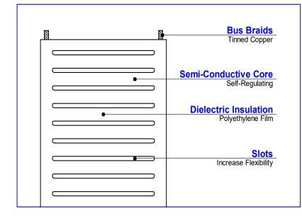
The STEP<sup>®</sup> Roof Deicing elements MEP-30-36W, MEP-23-36W, MEP-15-33W and MEP-7-33W are designed to prevent ice damming on roofs. The element is constructed of two parallel bus braids embedded in semi-conductive PTC polymer.
