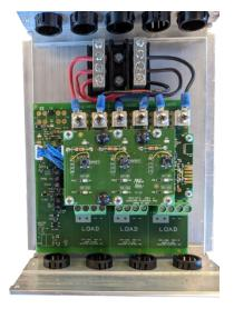
Picture of the DC Controller with one Main PCB and 3 channels.
