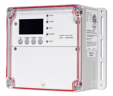
The S1 is a single-circuit IoT heat trace controller for use in snow melting, freeze protection and temperature maintenance applications. The device can drive up to a 30A resistive load to control electric heat trace systems operating between 120 VAC and 277 VAC. The S1 comes in an outdoor-rated enclosure tested to IP67 & NFMA 4X standards.
